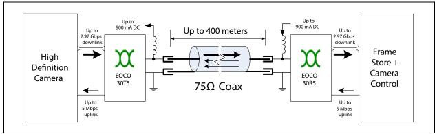
The EQCO30T5 includes an uplink receiver for receiving digital data coming from the frame store in full-duplex, giving 5 Mbps of bandwidth for:
