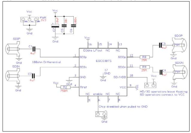
Resistors R8 and R9 are to be placed close to pins 12 and 11, respectively. From there onwards, the traces up to the coax connectors should be laid-out as  $75\Omega$  traces (including the C3 and C4 capacitors as AC-couplers).
